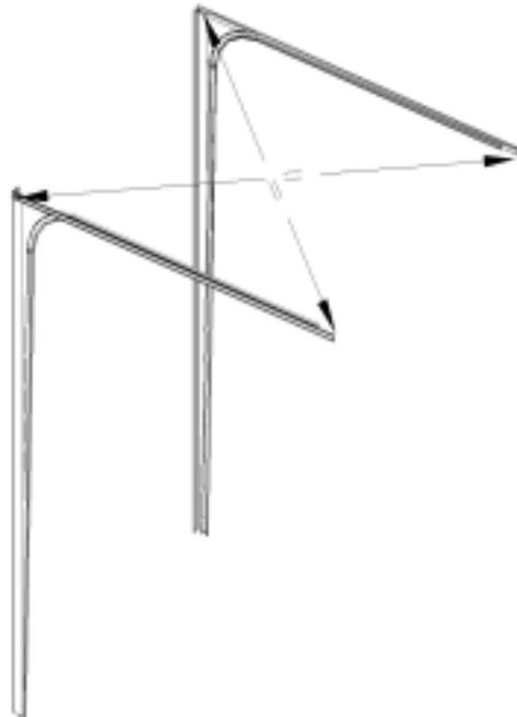
Secure further in this position the suspension of the horizontal track set.
